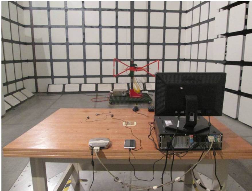
Radiated Emissions – Front View (Below 1 GHz)
