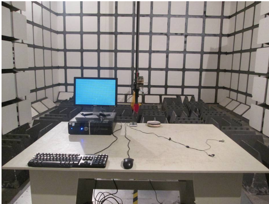
Radiated Emissions – Front View (Above 1 GHz)
