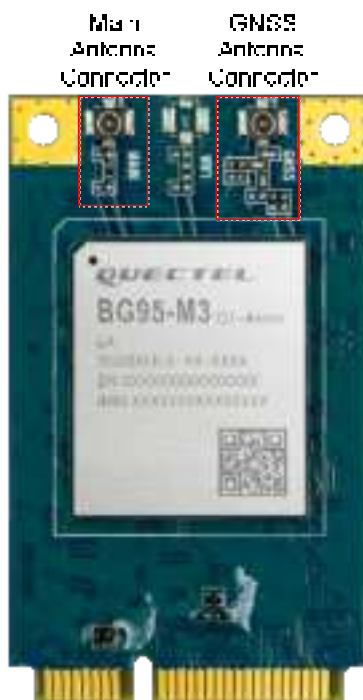
Figure 13: Main and GNSS Antenna Connectors
