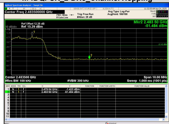
Out Of Band Emission(Right) \pi/4 DQPSK_2-DH5_Channel Hopping
