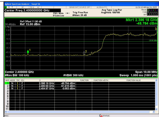
Out Of Band Emission(Left) \pi/4 DQPSK_2-DH5_Channel Hopping
