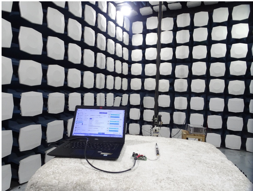
Picture 1 Radiated Emission Test Setup
