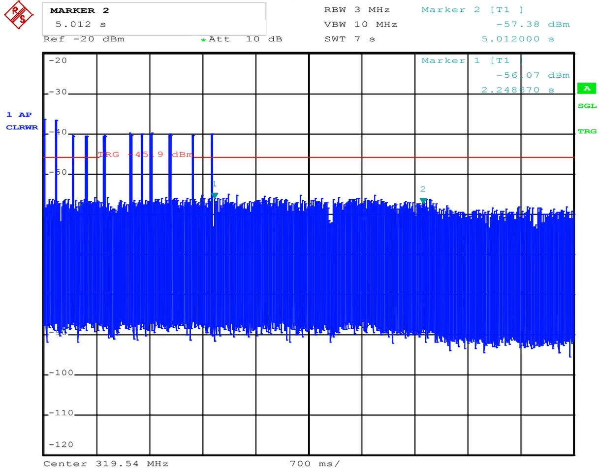
Pulse train exceeds 100ms, so duty cycle correction factor is calculated based on 100ms window
