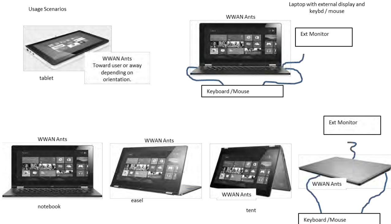
After a review of the usage scenarios displayed above, the following positions were tested for the WLAN radio: right edge, left edge, and back side adjacent to the antennas. Each of these positions was tested with the keyboard folded under the display ("tablet mode") or extended away from the display ("tent mode").
