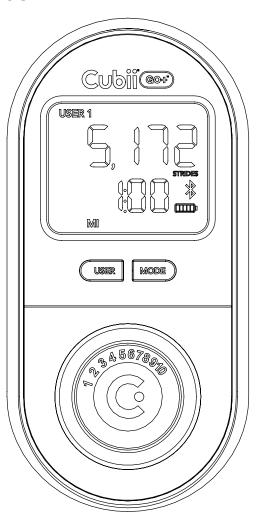
Press the MODE button to switch which metric is displayed. You can use the SCAN mode to automatically toggle between the above metrics every 7 seconds. The triangle indicator shows which view is selected.
