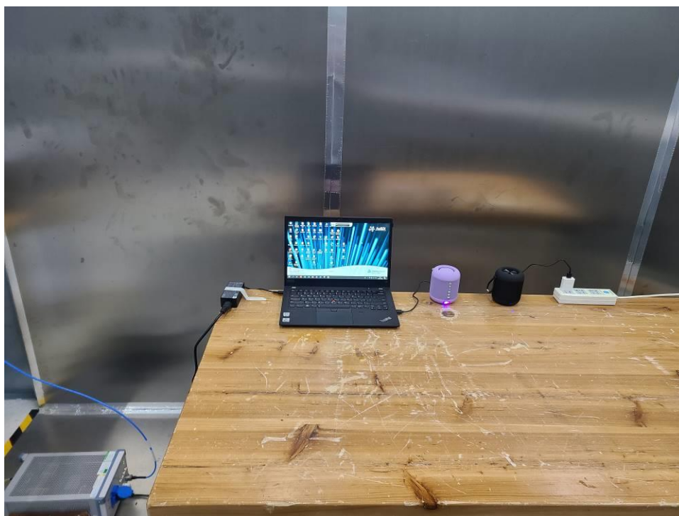
Photograph 1: Set-up for Conducted Emission on AC Mains
