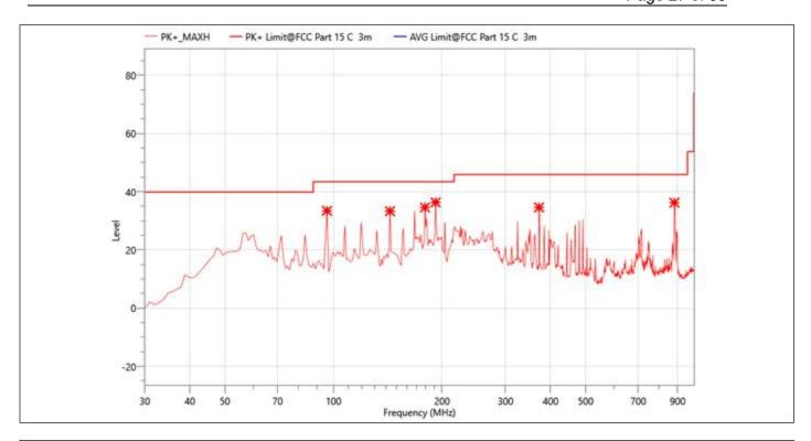
Site: ChamberA-2 Antenna: Vertical Temperature(C):23(C) FCC Part 15 C 3m Radiation(QP) Limit: Humidity(%):57% EUT: 2023-05-12-03 WIFI BT module **Test Time:** M/N.: 6252B-PR **Power Rating:** DC 5V TX2402 **Test Engineer:** Mode: Luffy Note:
