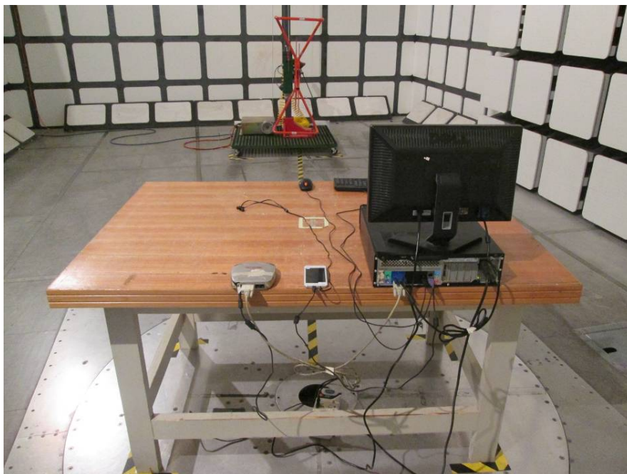
Radiated Emissions – Rear View (Below 1 GHz)
