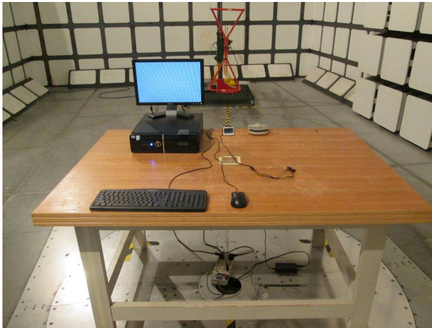
Radiated Emissions – Front View (Below 1 GHz)
