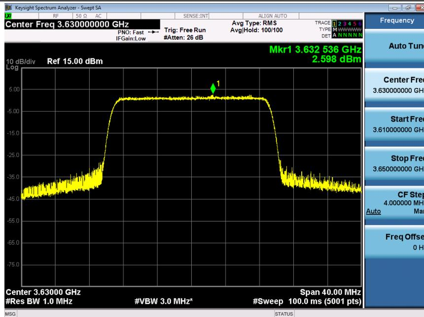
$EIRP\ PSD = 2.598 - 6.12 + 4.5 = 0.978\text{ dBm/MHz}$ , Antenna gain is  $-6.12\text{ dBi}$ , the path loss is  $4.5\text{ dB}$
