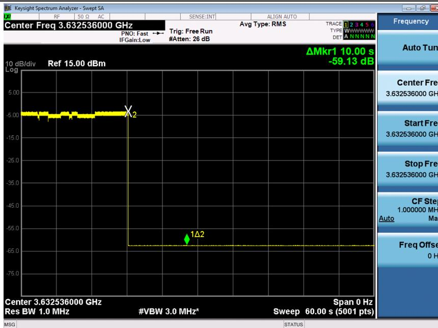
[Step 6] Setup with frequency 3650-3670MHz and power level 8dBm/MHz
