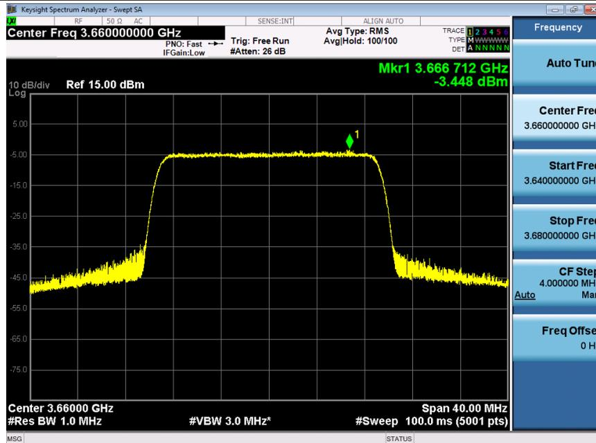
EIRP PSD=-3.448-6.12+4.5=-5.068dBm/MHz, Antenna gain is -6.12dBi,the path loss is 4.5dB
