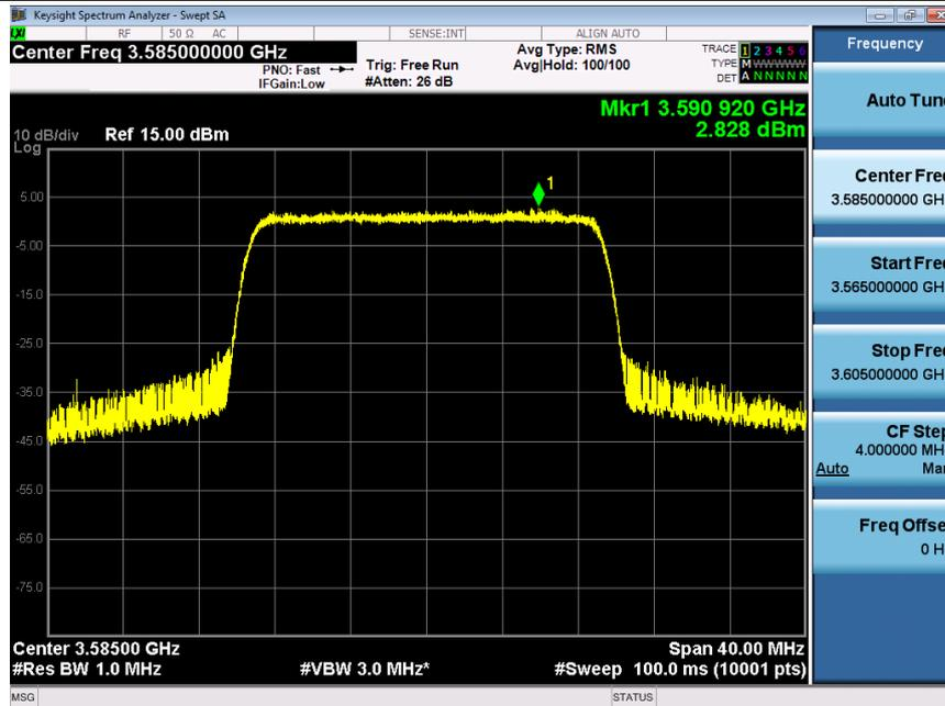
EIRP PSD=2.828-6.12+4.5+3=4.208dBm/MHz, Antenna gain is -6.12dBi,the path loss is 4.5dB, the MIMO Factor is 3dB
