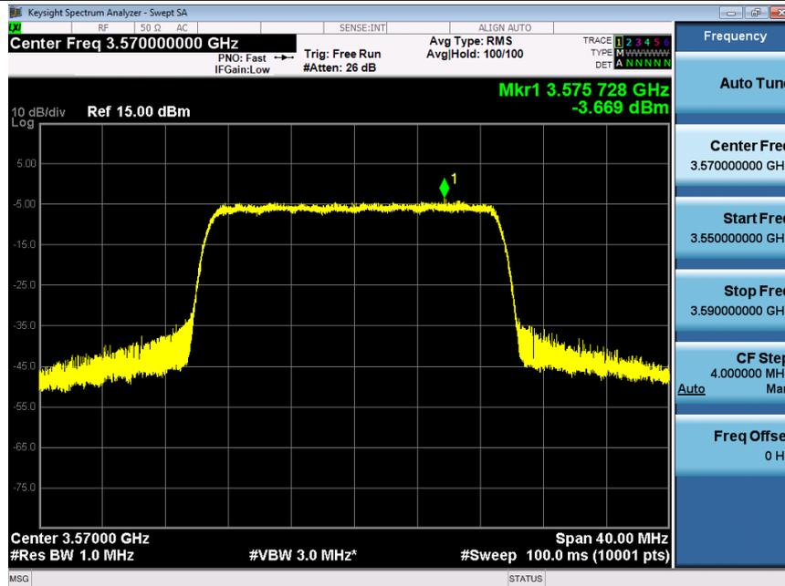
EIRP PSD=-3.669-6.12 +4.5+3=-2.289dBm/MHz, Antenna gain is -6.12dBi,the path loss is 4.5dB, the MIMO Factor is 3dB
