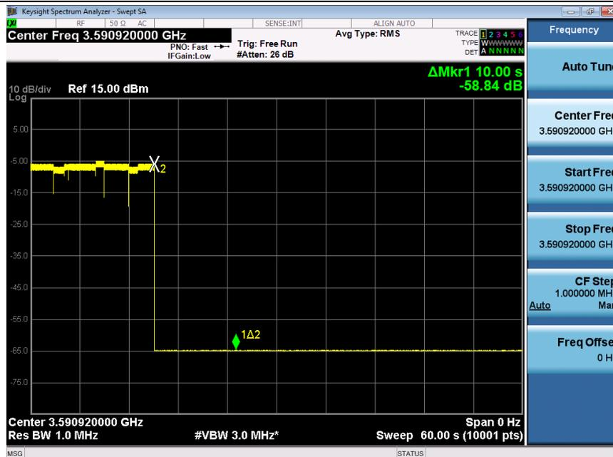
[Step 6] Setup with frequency 3560-3580MHz and power level 8dBm/MHz
