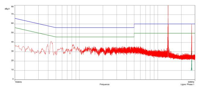
Class B of the standard FCC 47 CFR PART 15: 2017
