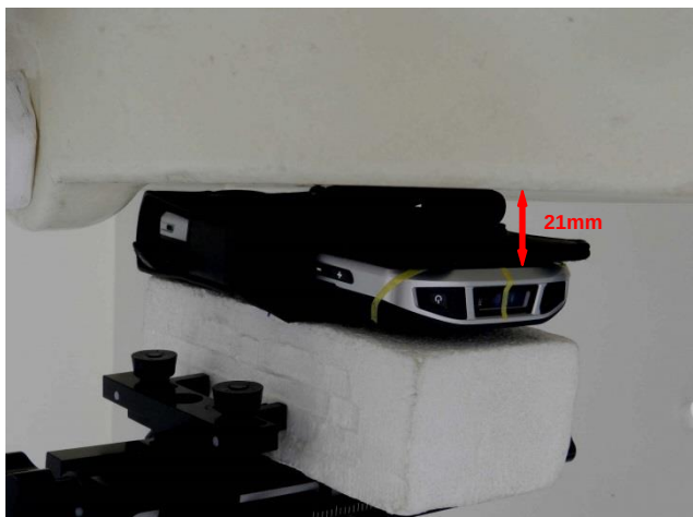
Front with Soft Holster, Test Separation 0 mm
