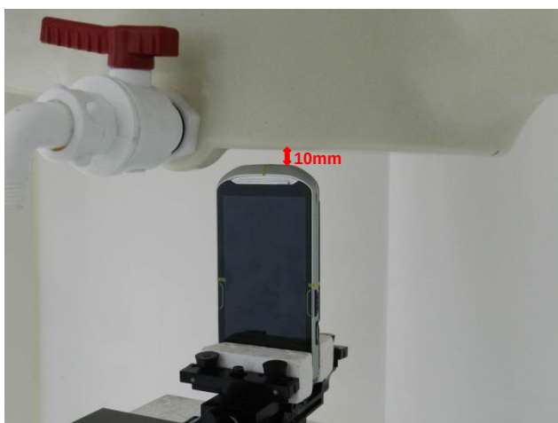
Bottom Side, Test Separation 10 mm
