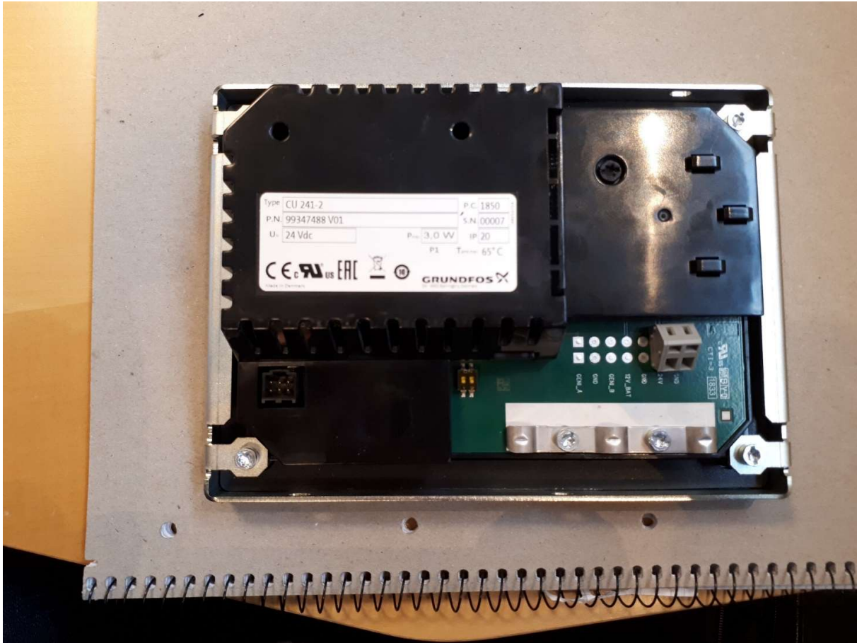
Figure 4 Position of label on backside of product. (Prototype unit, label information not correct)
