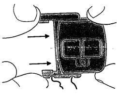
TO INSTALL PENDANT HOLDER, SLIDE HOLDER INTO SLOTS ON ENDS OF TRANSMITTER
