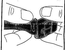
INTO SLOTS ON ENDS OF TRANSMITTER TO INSTALL WRISTBAND, SLIDE STRAPS
