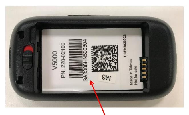
Label will be placed here inside battery compartment
