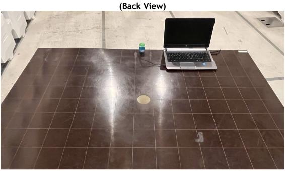
The EUT is placed at the center of the turn table
