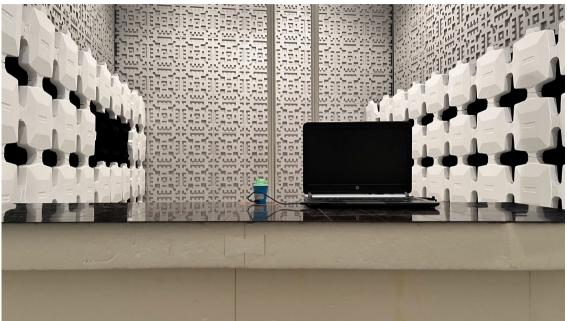
The EUT is placed at the center of the turn table
