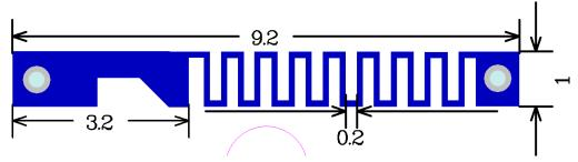
Antenna Type: PCB Antenna
