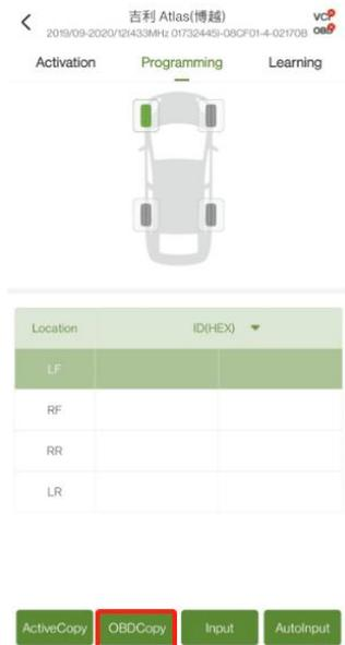
Step 6: Put the sensor close to the VCI and write the new ID
