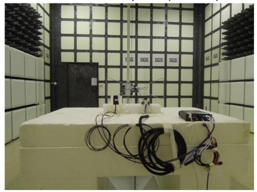
Radiated Emission Set up Photos (Above 1GHz)
