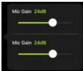
*The top slider adjusts gain for first mic and the bottom slider adjusts mic gain for the second*
