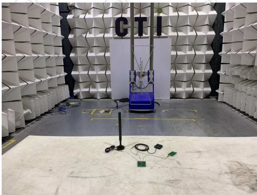
Radiated spurious emission Test Setup-1(Below 1GHz)
