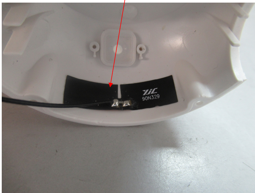
EUT – Wi-Fi Antenna View
