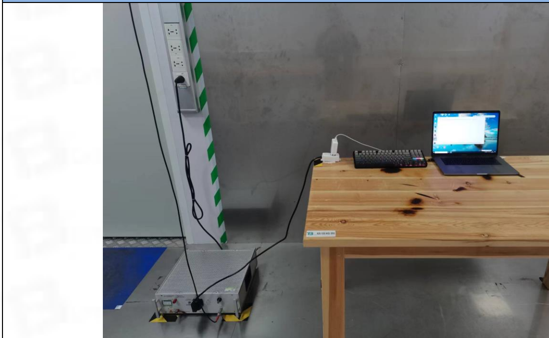
Conducted Emission at AC power line
