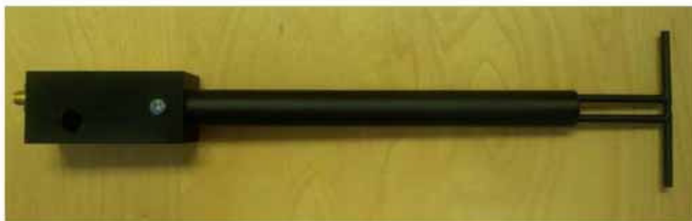
Figure 1 – MVG COMOSAR Validation Dipole
