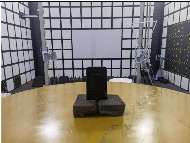
Spurious Radiated Emissions Test setup
