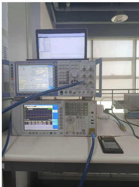
'RF Conducted Test setup (GSM/WCDMA/LTE)
