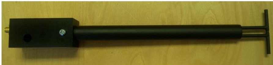
Figure 1 – MVG COMOSAR Validation Dipole
