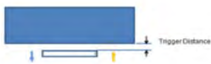
Picture : Proximity sensor triggering distances assessment(Back/front side)
