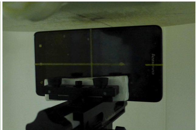
Left Side of the DUT with Phantom 1 cm Gap
