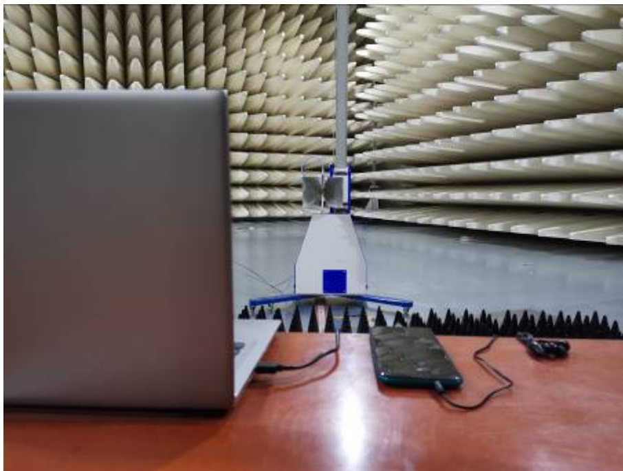
Radiated Emissions Test Setup (above 1GHz)
