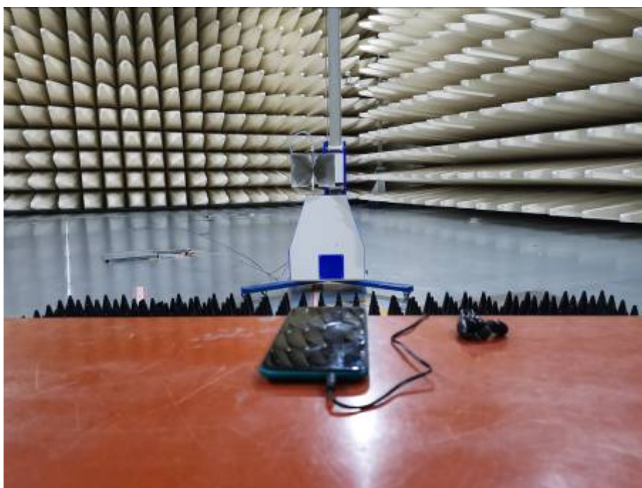
Radiated Emissions Test Setup (above1GHz)
