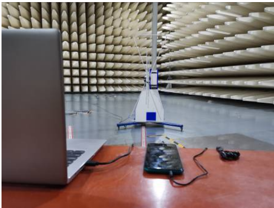
Radiated Emissions Test Setup (30-1000MHz)
