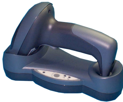
Charging the Batteries
