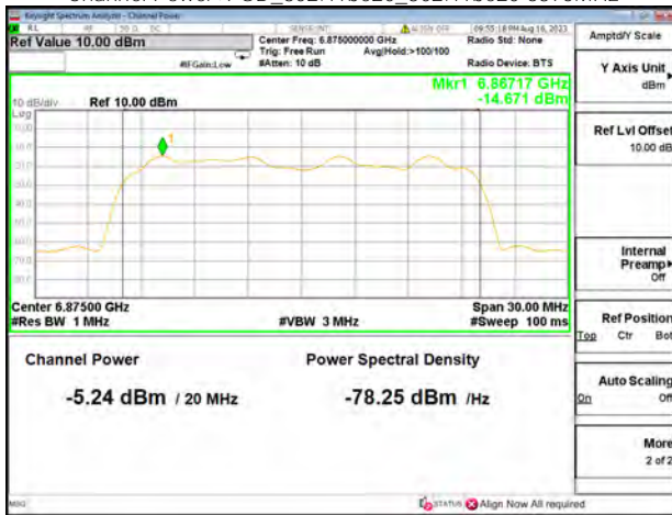
Channel Power+PSD_802.11be20_802.11be20 6895MHz
