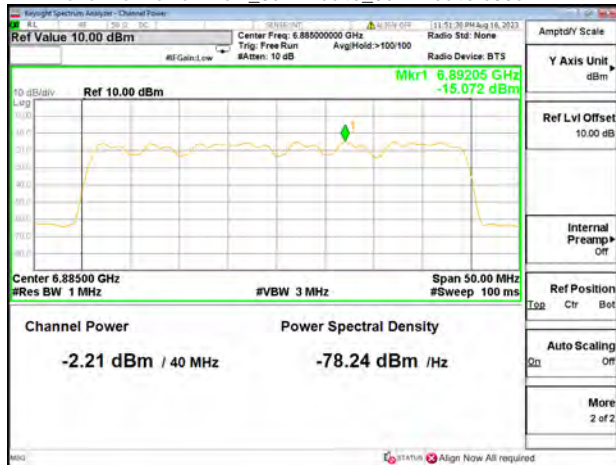
Channel Power+PSD_802.11be40_802.11be40 6925MHz
