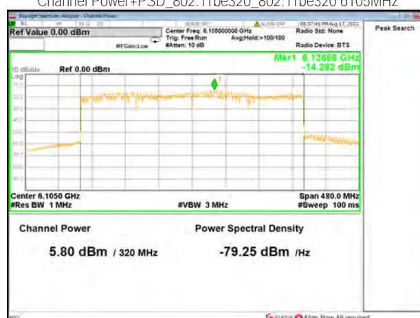
Channel Power+PSD_802.11be320_802.11be320 6105MHz
