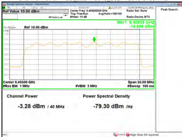
Channel Power+PSD_802.11be40_802.11be40 6445MHz
