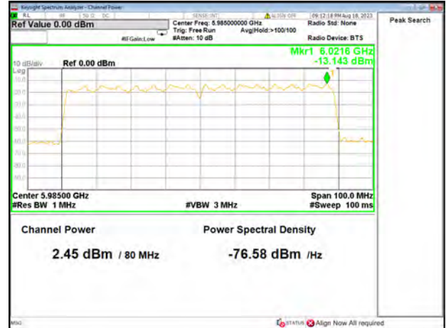
Channel Power+PSD_802.11ac80_802.11ac80 6145MHz
