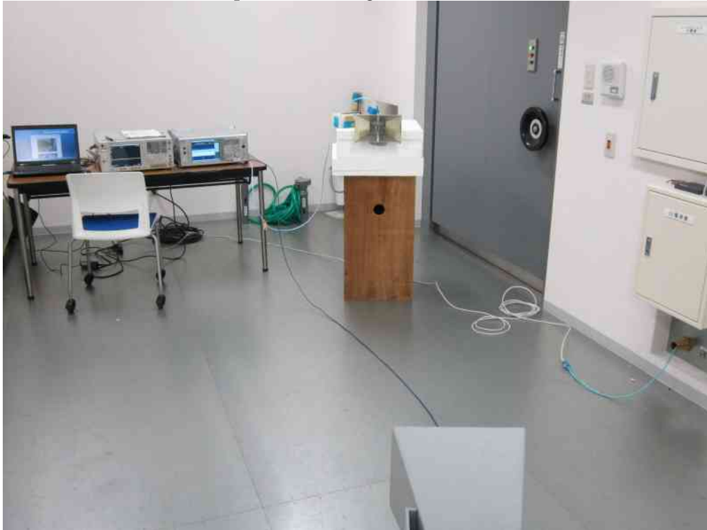
Test Setup for Generating the Radar Waveform
