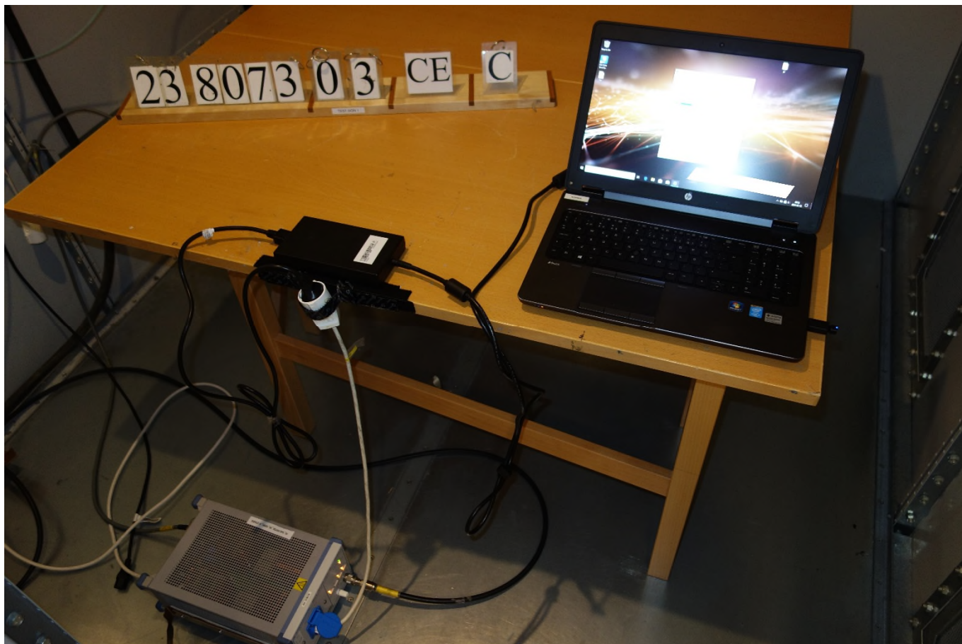
Test setup picture in Conducted Emission chamber
