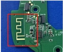
The antenna is PCB antenna. The best case gain of the antenna is -1 dBi.
