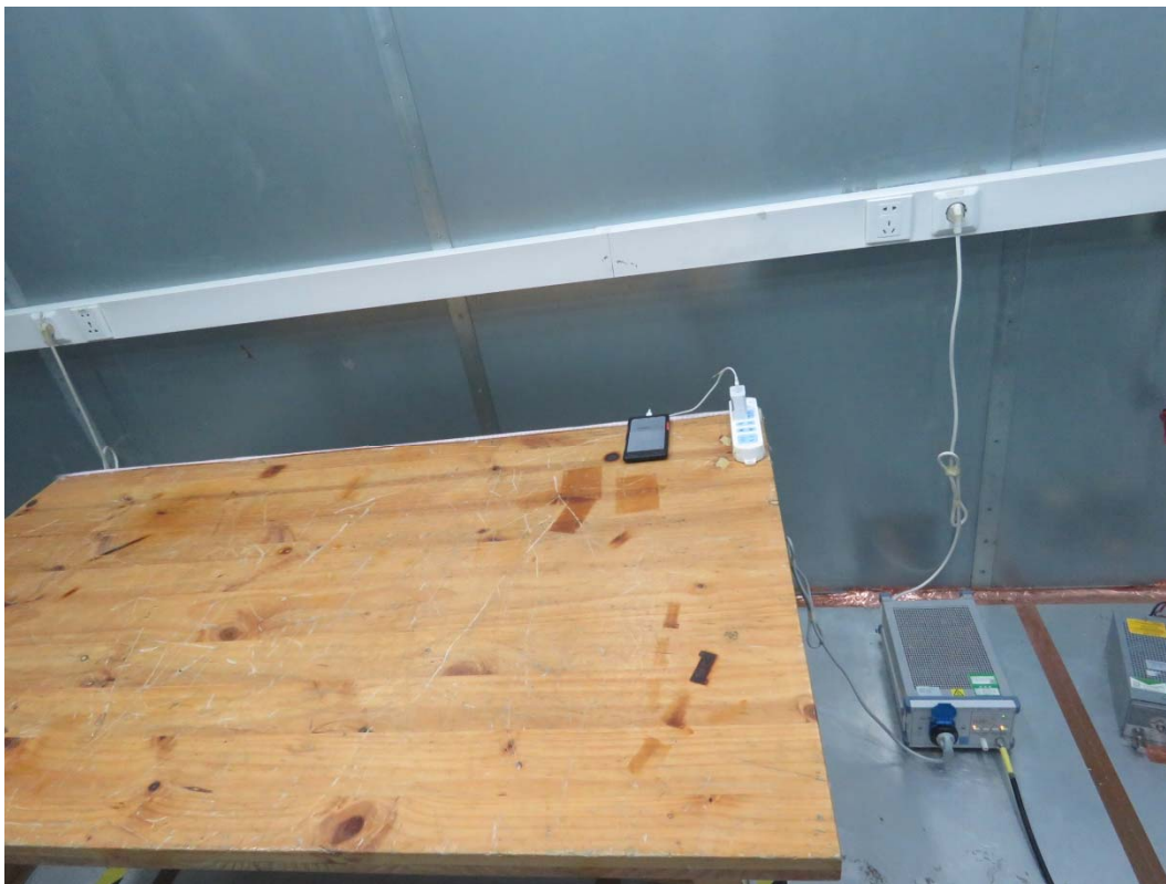
Picture 2 Conducted Emission Test Setup
