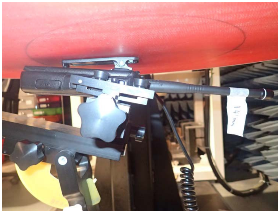
< Belt Clip Touch Position FA-S67VC 165MHz, BP-283 battery pack >
