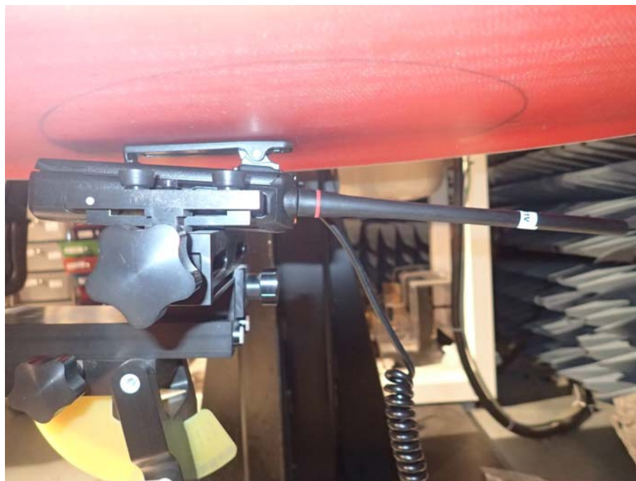
< Belt Clip Touch Position FA-S81V, FA-S82V, FA-S83V Antenna, BP-283 battery pack >
