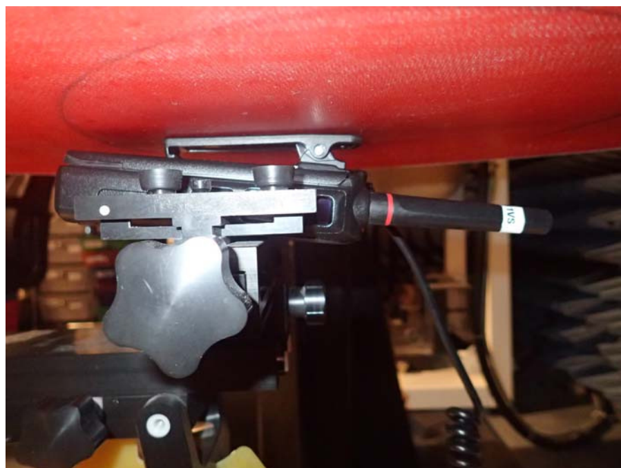
< Belt Clip Touch Position FA-S81VS, FA-S82VS, FA-S83VS Antenna, BP-283 battery pack >
