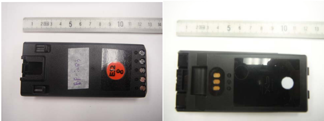
Li-ion Chargeable Battery (M/N: BP-283 Li-ion, 7.2V, 2010mAh)
