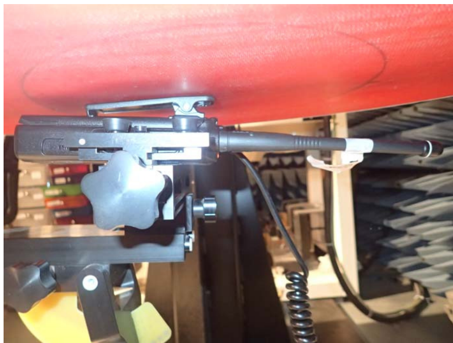
< Belt Clip Touch Position FA-S67VC 155MHz, BP-283 battery pack >
