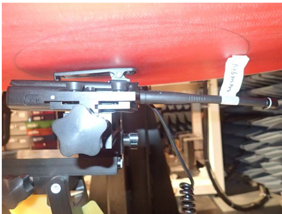
< Belt Clip Touch Position FA-S67VC 160MHz, BP-283 battery pack >
