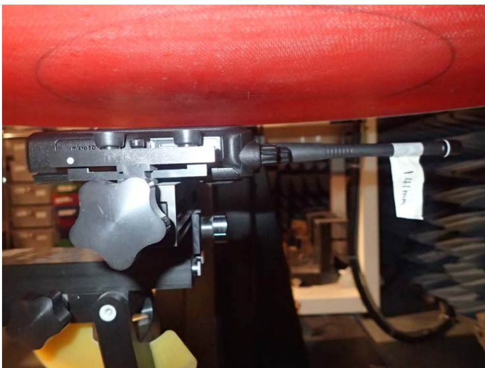
<Face Frontal Position, FA-S67VC 165MHz, BP-283 battery pack>
