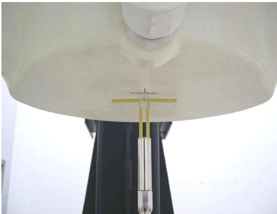
Picture 8.2 Photo of Dipole Setup
