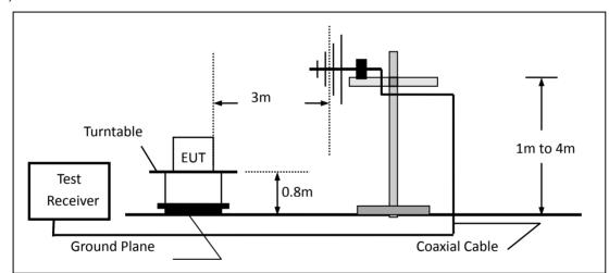
(c) For radiated emissions above 1000MHz
