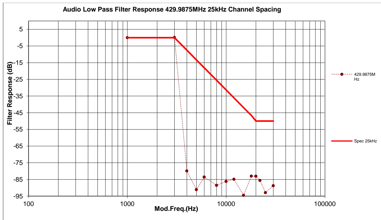
Figure 6C-2: 25 kHz Channel Spacing, 429.9875 MHz, Transmit Audio Low Pass Filter Response (Not for FCC review)
