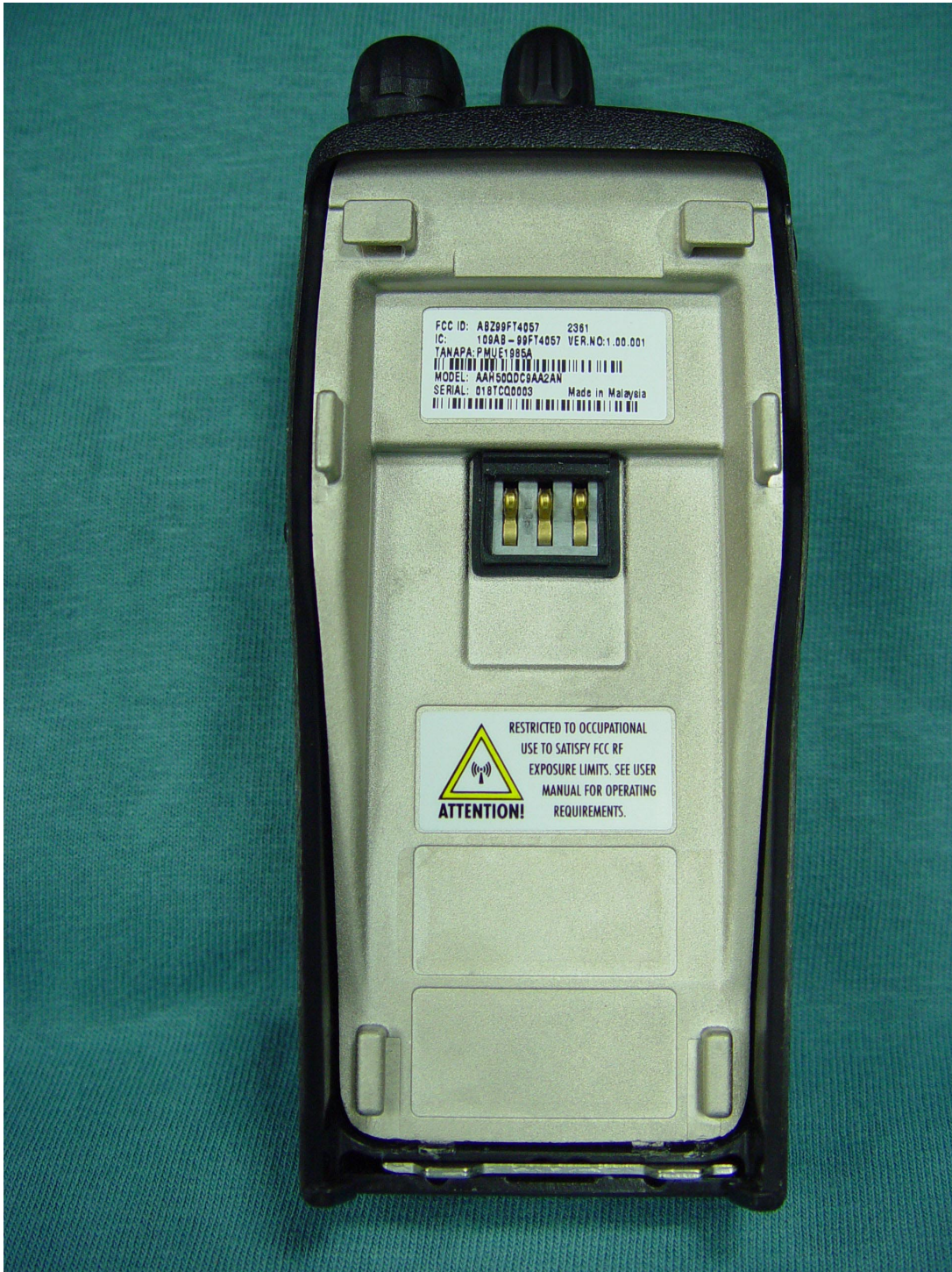
REAR VIEW WITH BATTERY REMOVED SHOWING FCC ID LABEL AND RF SAFETY LABEL
