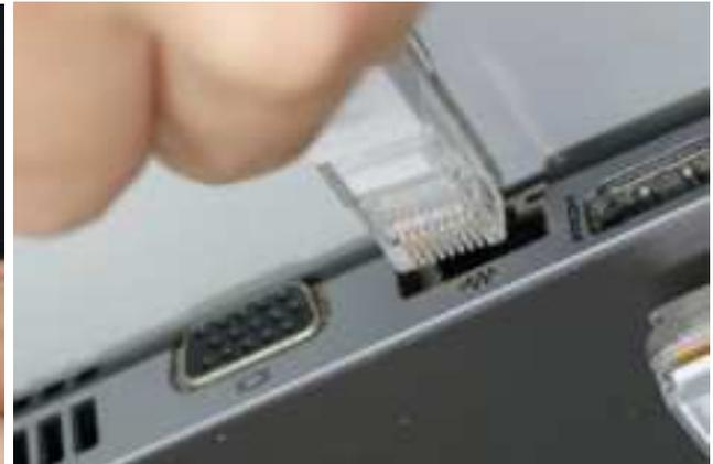
Plug one end of the supplied Cat 5E cable into the Access Point, the other end should be plugged into your computer.
