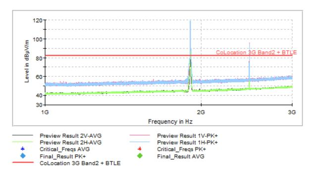
The peaks above the limit are the 3G Band II and the Bluetooth carrier frequencies.
