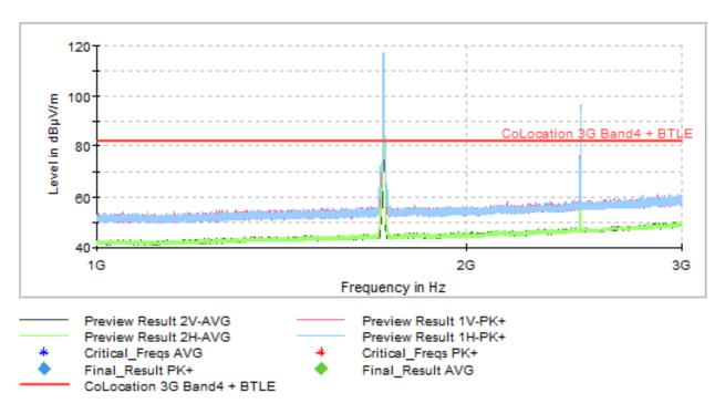
The peak above the limit is the 3G Band IV and the Bluetooth carrier frequency.
