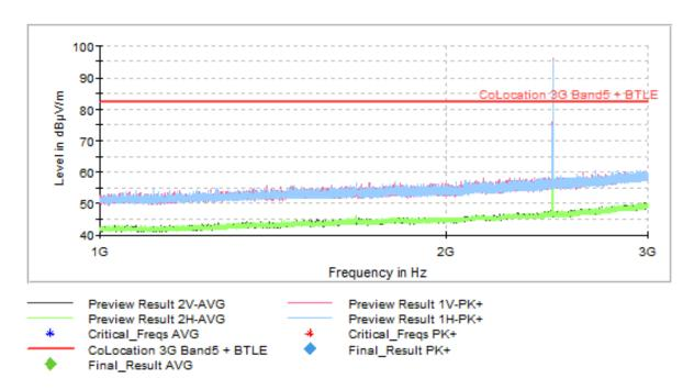
The peak above the limit is the Bluetooth carrier frequency.
