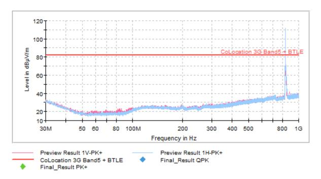
The peak above the limit is the 3G Band V carrier frequency.
