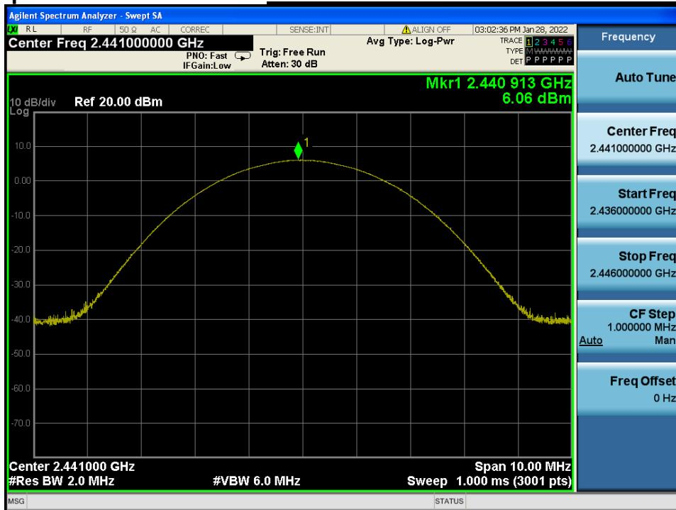
**Peak Output Power****Highest Channel & Modulation : 8DPSK**
