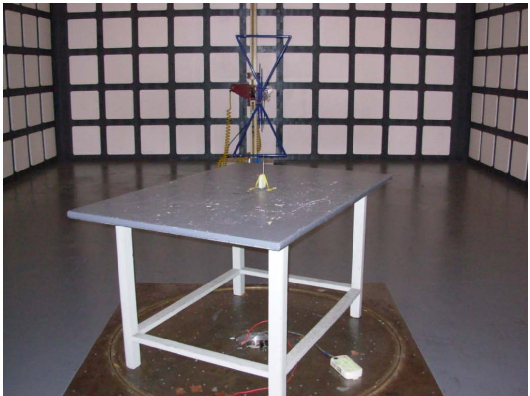
SETUP WITH MAXIMUM DETECTED EMISSION AT VERTICAL POLARIZATION (FOR ON STAND TEST MODE)
