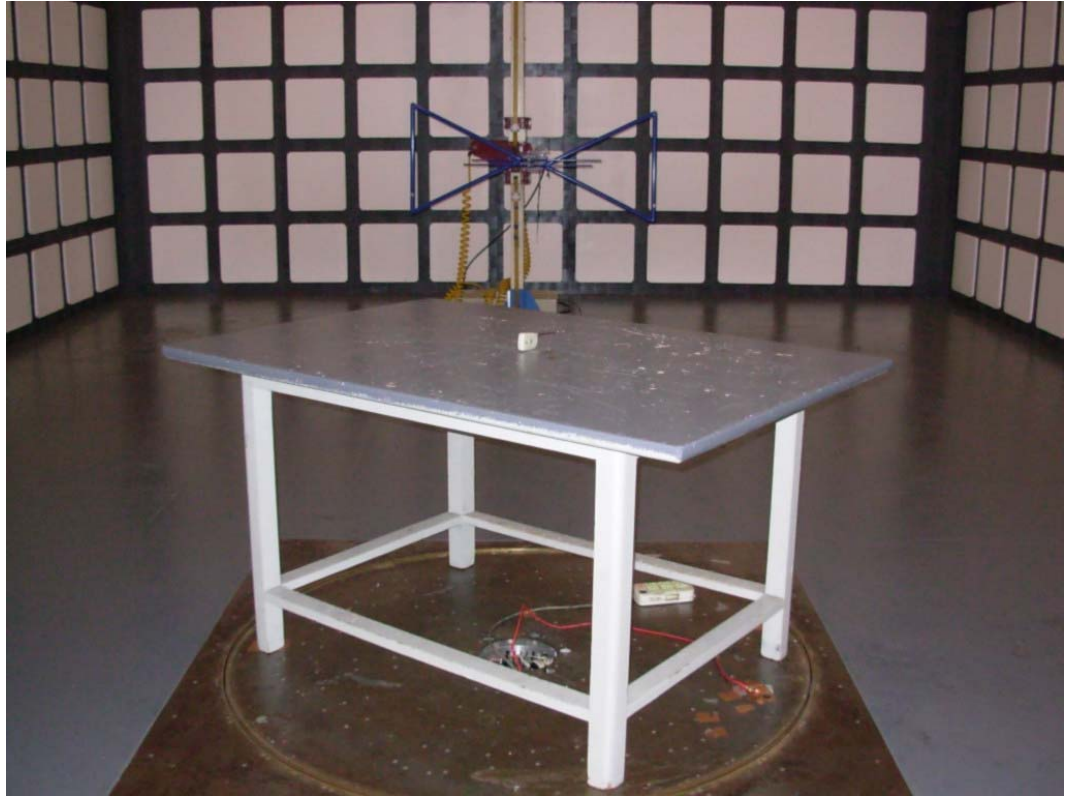
SETUP WITH MAXIMUM DETECTED EMISSION AT HORIZONTAL POLARIZATION (FOR ON SIDE TEST MODE)
