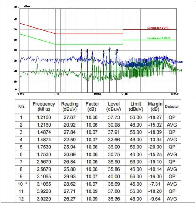
1.An initial pre-scan was performed on the line and neutral lines with peak detector.
