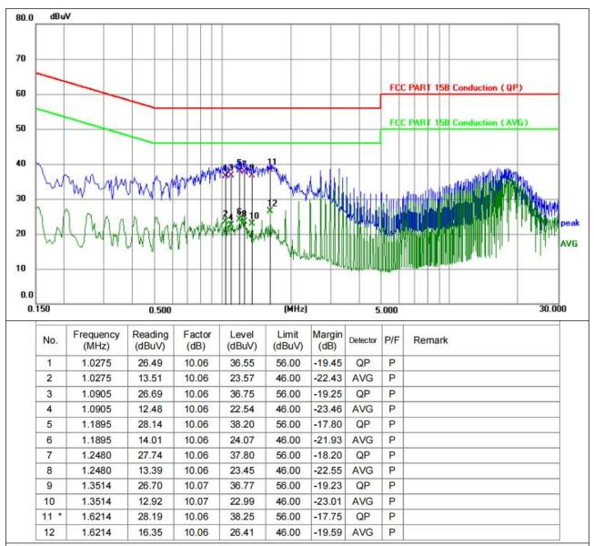
1.An initial pre-scan was performed on the line and neutral lines with peak detector.
