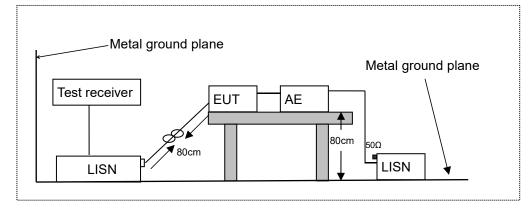
LISN: Line Impedance Stabilization Network AE: Associated equipment EUT: Equipment under test
