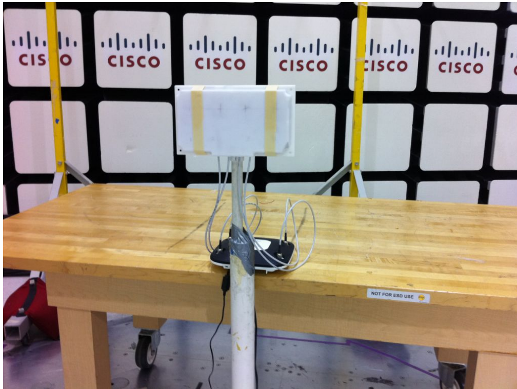
2.4/5 GHz Dual Band 6dBi MIMO patch antenna
