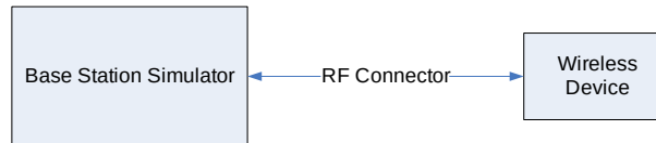
Figure 9-3 Power Measurement Setup
