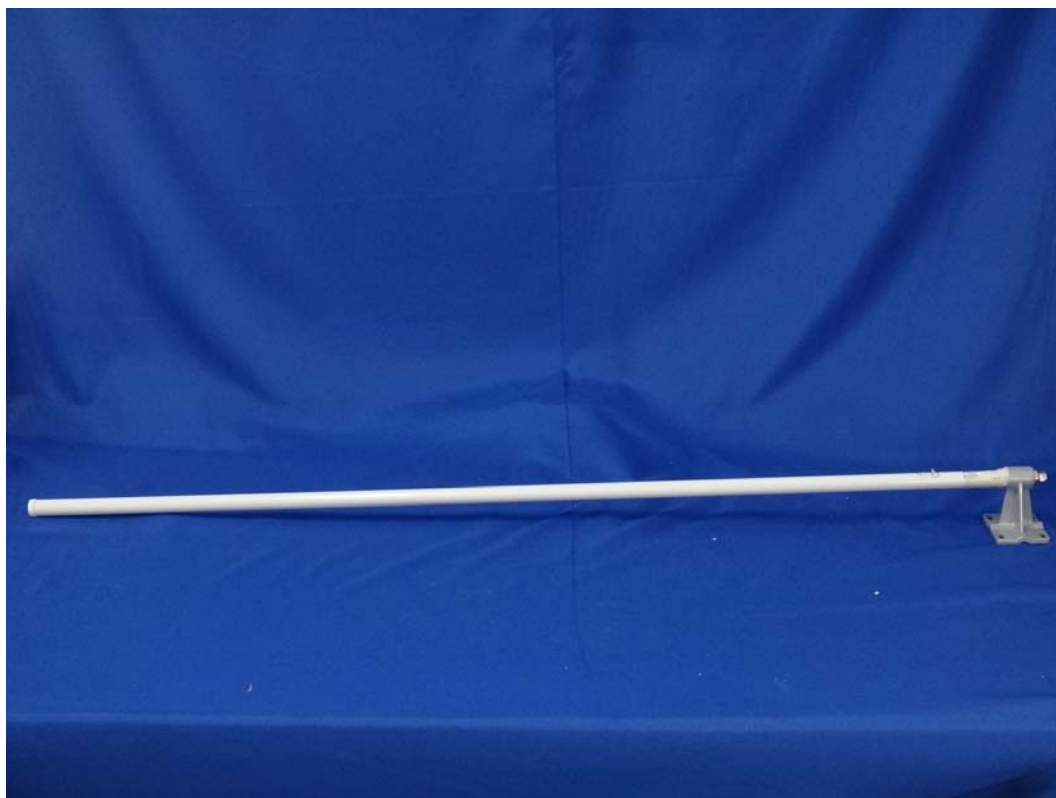
(14) EUT Photo (Omni Antenna)
