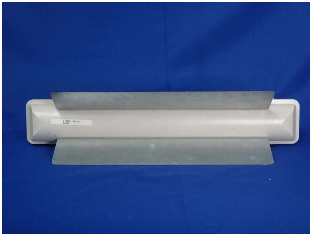
(12) EUT Photo (Sector Antenna)
