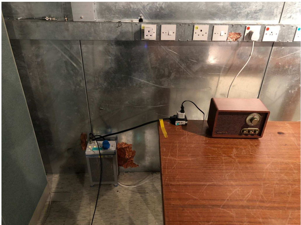
Set-up for AC power line Conducted Emission
