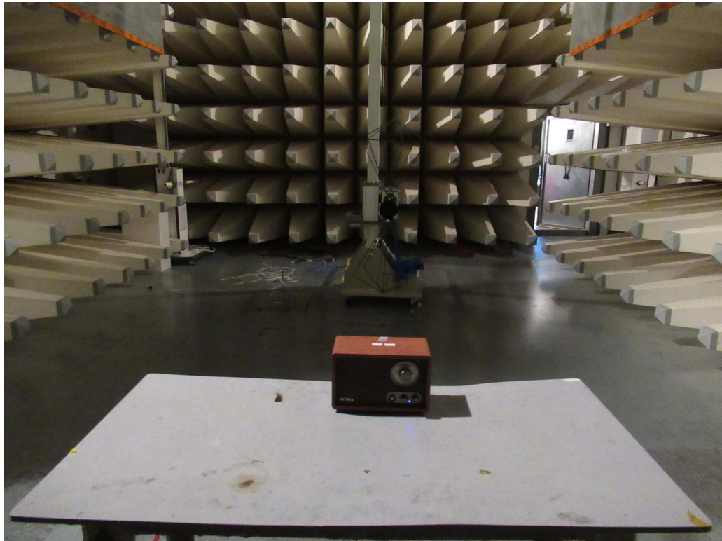
Set-up for Radiated Emission
